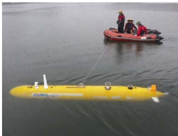
Figure 11—Surface Test of ISiMI6000
