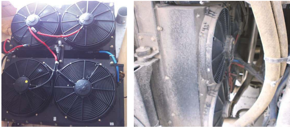
FIGURE 10: Actual fan and on-vehicle configurations for driving test.
