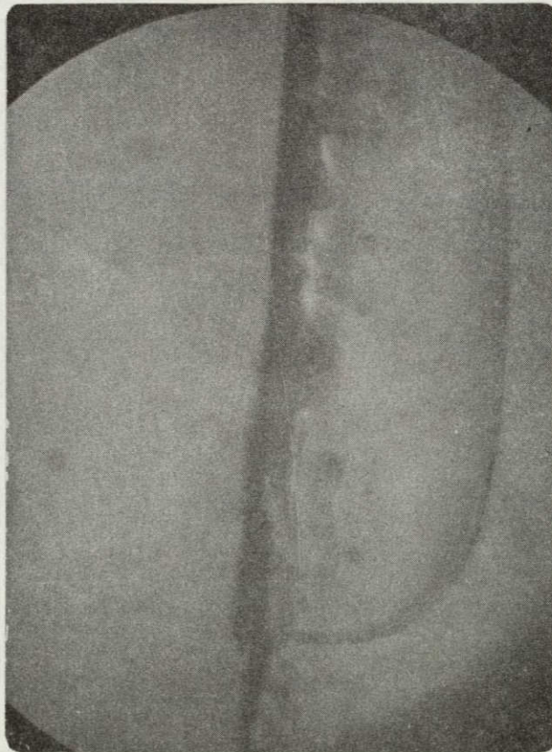
Figure 2.2-5 UNACCEPTABLE HOT WIRE BECAUSE OF GLASS CHIP (50x) CELL ON RIGHT SIDE.
