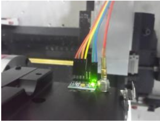
Figure 2 – Accelerometers mounted on the spindle housing; MPU6050 (Left), Dyatran 3145AG (Right)
