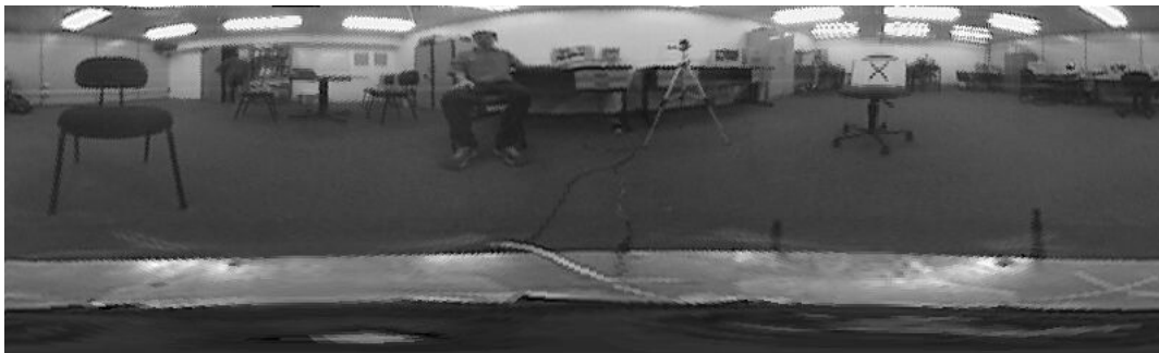
Figure 13. Panoramic image created by a direct mapping of the pixels of the image acquired by the spherical mirror.
