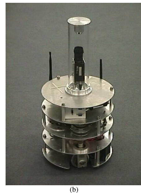
Figure 11. (a) Omnidirectional vision system prototype with hyperbolic mirror and (b) mobile robot with omnidirectional vision system.
