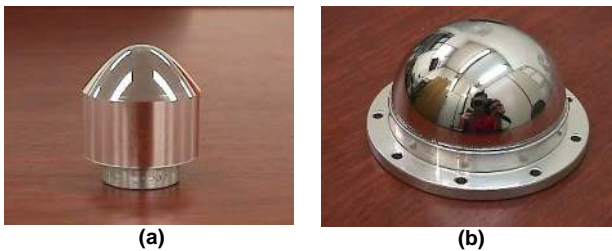
Figure 10. Convex mirrors built. (a) Hyperbolic mirror with 40 mm of diameter machined on aluminum by an ultraprecision CNC lathe. (b) Spherical mirror with 70 mm of diameter built using glass.
