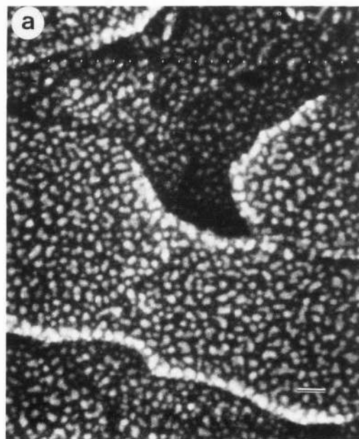
Fig. 8. Resolution test sample; (a) Pt sputter coated on carbon, taken at 30 kV. Bar = 10 nm. (b) Au-Pd sputter coated on carbon, taken at 1 kV. Bar = 100 nm. Specimens were heated at 150°C during photographing (50 sec/frame) to avoid contamination.
