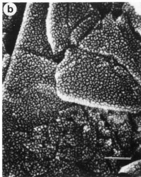
Fig. 8. Resolution test sample; (a) Pt sputter coated on carbon, taken at 30 kV. Bar = 10 nm. (b) Au-Pd sputter coated on carbon, taken at 1 kV. Bar = 100 nm. Specimens were heated at 150°C during photographing (50 sec/frame) to avoid contamination.
