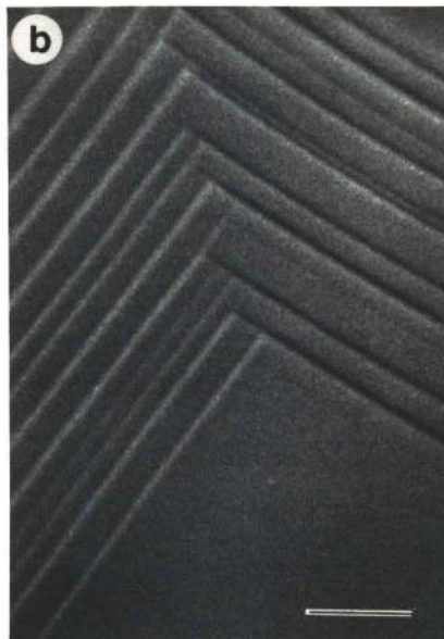
Fig. 10. Direct observation of MgO; (a) and (b) crystal step taken at 10kV, bar = 100nm; (c) a small cubic crystal (bar = 20nm) attached to a large crystal shown in (d); (d) bar = 200nm; (e) direct carbon replica taken by TEM, bar = 20nm.
