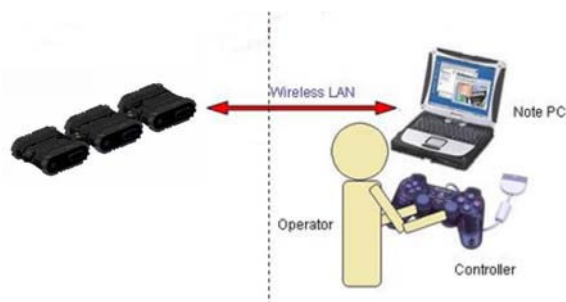
Fig. 4. Control system of KOHGA2
