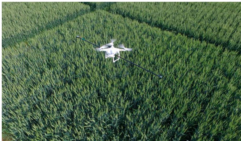
Figure 12. Field tests based on UAV-borne crop-growth monitoring system.
