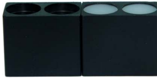
Figure 4. The lightweight structure used for the multispectral crop growth sensor.
