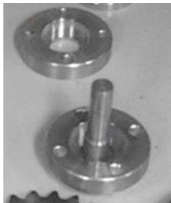
Figure 6. The brackets hold bearings and waterproofing the chassis.
