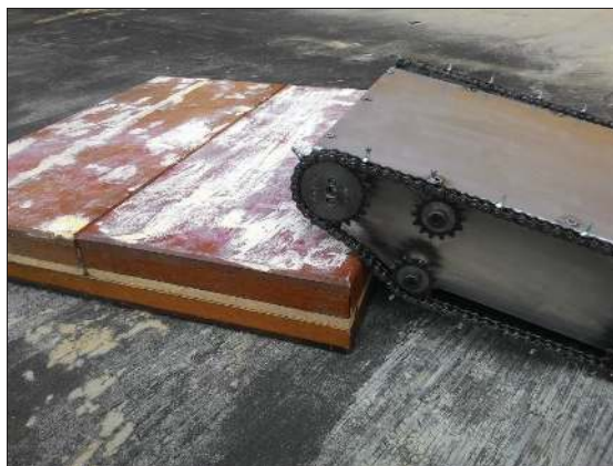
Figure 12. The crawler climbed the 9.5 cm obstacles.
