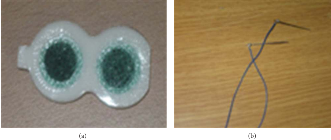
FIGURE 3: (a) Uni-Patch Tyco EMG electrodes (b) needle-type conductive electrodes.
