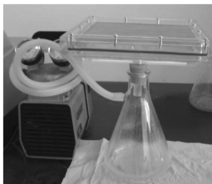
Fig. 1. Schematic diagram of filtering apparatus for preparing of Hanji fiber sheet.
