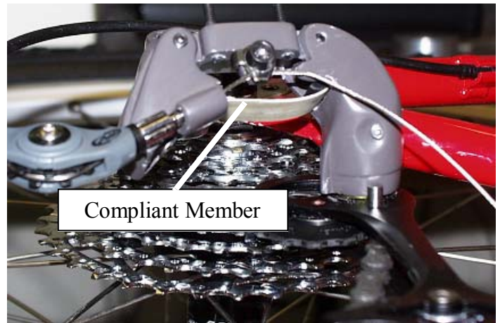
Figure 10. Final prototype for a fully re-tooled derailleur
