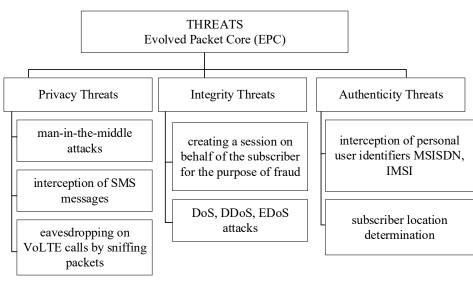
Fig. 4. Main types of attacks on Evolved Packet Core
