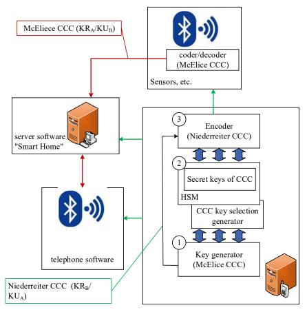
Fig. 8. Block diagram of a two-circuit security system of the "Smart Home" system based on CCC
