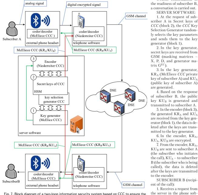
Fig. 7. Block diagram of a two-loop information security system based on CCC to ensure the confidentiality of voice messages
