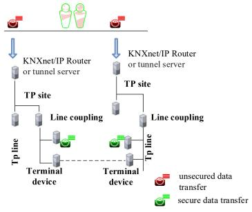
Fig. 2. Security in mobile wireless channels based on KNX
