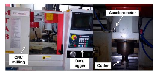
Figure 2. The schematic of the experimentation arrangement.
