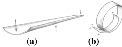
Figure 4-10. Bi-stable arched metal strip used in slap bracelets. By deflecting the center of the strip (a), it collapses into its other (coiled) stable equilibrium position.
