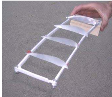
Figure 4-22. In-plane bending prototype from Figure 4-11 with airfoil-shaped ribs added. Rib action during deployment is illustrated in Figure 4-23.
