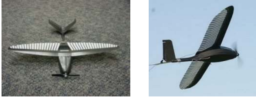
Figure 2-16. The flexible composite airframe built by the USAF and University of Florida. [25]
