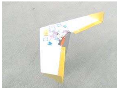
Figure 5-17. IRIS, BYU's 45 cm wingspan 'flying wing' UAV.
