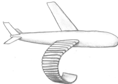
Figure 4-6. A segmented rolling wing, shown rolling up without a second layer for stiffening.
