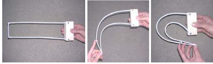
Figure 4-12. Hardware demonstrating in-plane bending of a wing. The model uses 5 mm thick polypropylene rods pinned to a wooden block.
