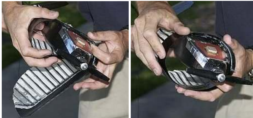
Figure 2-17. The airframe is stored by (a) bending the wings down and (b) curling them around the fuselage. [25]
