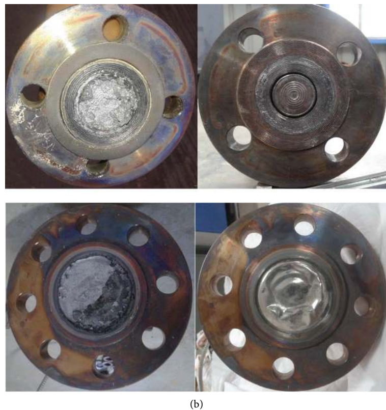
Figure 9. (a) Long duration test data for NaK fill fluid based and silicone oil fill fluid based pressure sensors on Pb-Li (gradual changes in applied pressure represent decrease of pressure with time). M-shaped cycles at the start and end of long duration test represent calibration cycles from 0 to 1 MPa (g) and vice-versa; (b) Condition of wetted diaphragm seals for NaK fill fluid based and silicone oil fill fluid based pressure sensors after over 1000 hour continuous exposure to liquid Pb-Li and after chemical cleaning.
