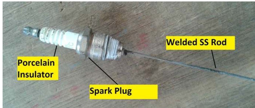
Figure 3. Conductivity level switch construction.
