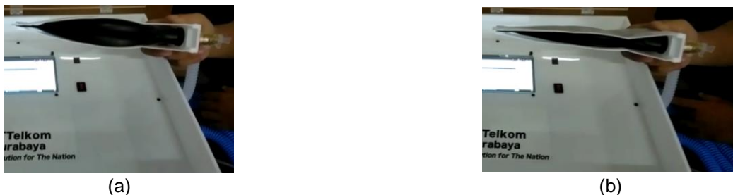
Figure 5. Digital Ventilator Testing using Test Lung: (a) Test Lung Expanded During Respiration; (b) Test Lung Retracted During Expiration
