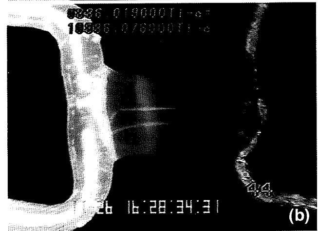
Fig. 14. Crystallization behavior of simulated mold slags. (a) 50°C/s (3.8% Na 2 O, 6.8% Al 2 O 3 , C/S=1) (b) 80°C/s (5% Na 2 O, 6.7% Al 2 O 3 , C/S=1)
