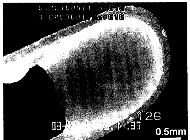
Fig. 15. Crystallization behavior of industrial mold slag by SHTT in isothermal experiment for TTT diagram (1215°C).
