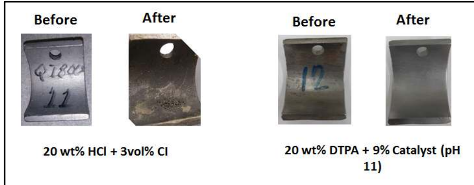
Figure 9 —Photographs for the casing coupons before and after the corrosion tests at 70 °C and 10340 kPa (1500 psi).
