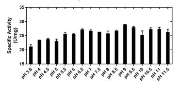
**Figure 7.** Specific activity (U/mg) of the bottom phase of ATPS in pH range of 3.6 to 11.5 using 2% (w/v) azocasein as substrate. The data represent the mean  $\pm$  SD (N = 3).
