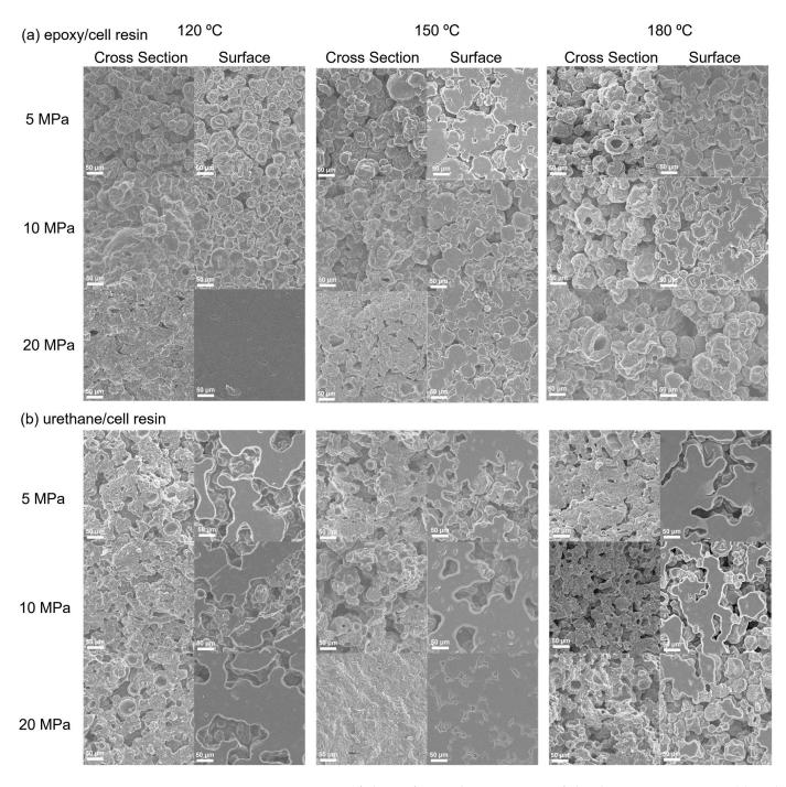
Figure 3. SEM images of the surface and cross section of the thermosetting epoxy– (a) and urethane–cell (b) resins.
