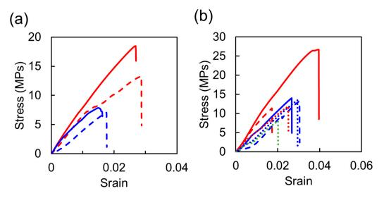
**Figure 4.** Typical stress–strain curves of the epoxy/cell (**a**) and urethane/cell (**b**) resins. The blue, red and green lines show the data of the resins formed at 120, 150 and 180 °C, respectively. The solid, dashed and dotted lines show the data of the resins formed at 20, 10 and 5 MPa, respectively.
