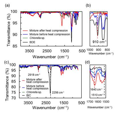
**Figure 2.** IR spectra of the thermosetting epoxy–cell (**a**,**b**) and urethane–cell (**c**,**d**) resins. Spectra enlarged for each wavelength region are shown in (**b**,**d**). The spectra of the mixture of monomer and *Chlorella* sp. After and before heat compression, *Chlorella* sp. and monomer are shown by red, blue, green and black lines.
