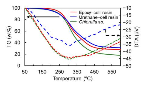
**Figure 5.** TG (solid lines) and DTA (dashed lines) curves of the thermosetting epoxy– (red) and urethane– cell resins (blue) and *Chlorella* (green). Solid and dashed arrows indicate TG and DTA data, respectively.
