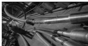
Figure 6 Smart cables based on FBGs
