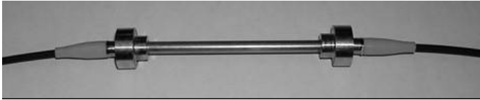
Figure 1 Picture of metal tube encapsulated FBG strain sensor
