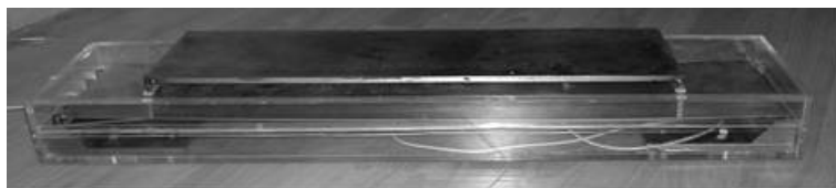
Figure 5 Structure of ice load sensing device based on dual FBG
