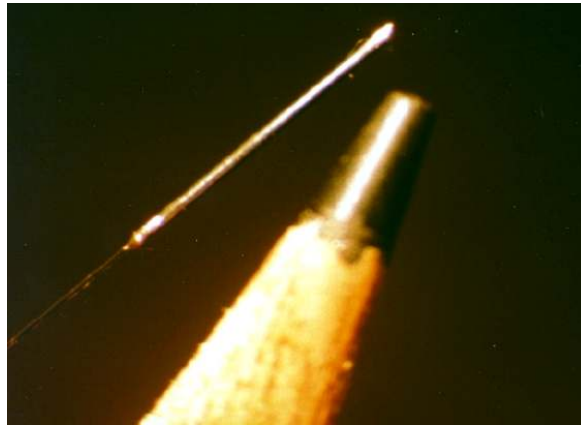
Figure 81. Photograph of fiber optic temperature sensor using metal wire.
