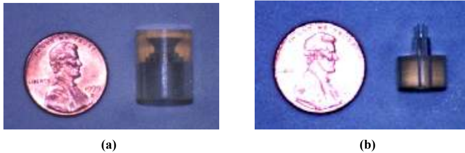
Figure 56. Photographs of the (a) top and (b) bottom pieces of the SLA gage
