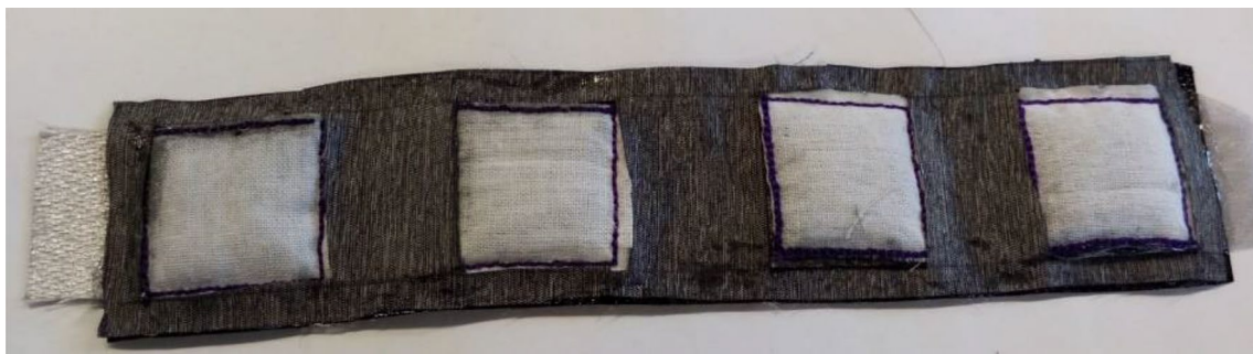
Fig. 3 Prototype of a multi-cell flexible textile Al-Air battery with cells arranged on a plane
