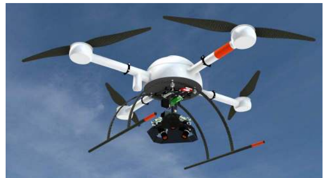
Figure 4: Schematic drawing of the UAV with newly developed multi head camera system "Four Vision"
