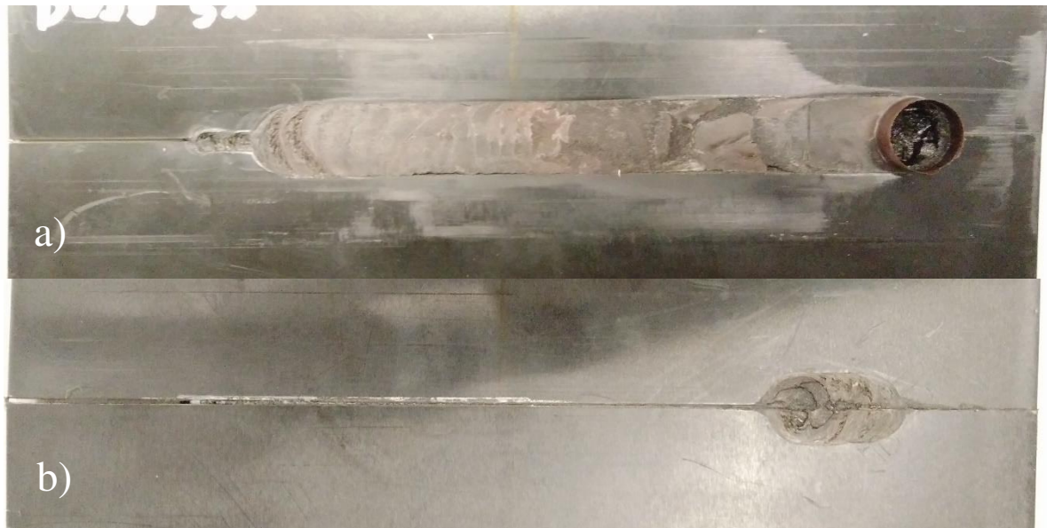
Figure 62 - Weld from hybrid tool preheated to 150 °C, a) top view, b) bottom view.
