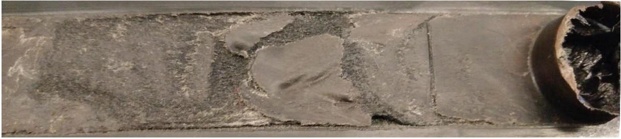
Figure 64 - End section of weld produced by hybrid tool preheated to 150 °C
