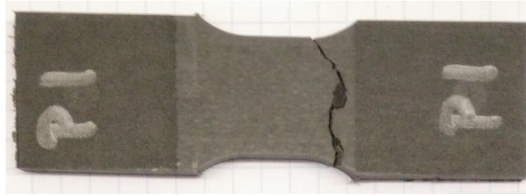
Figure 33 - Specimen P1 broken outside the gauge length
