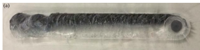
Figure 21 - Weld seam obtained using nonthreaded probe [40]
