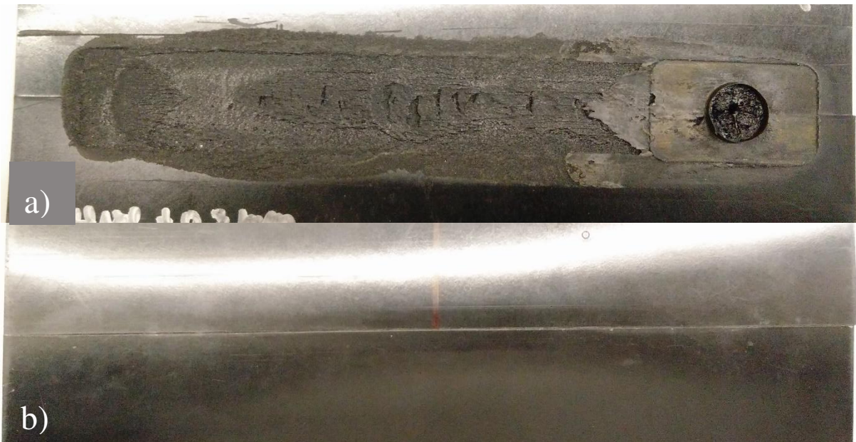
Figure 67 - Weld from hybrid tool with protruding sleeve preheated to 270 °C, a) top view, b) bottom view
