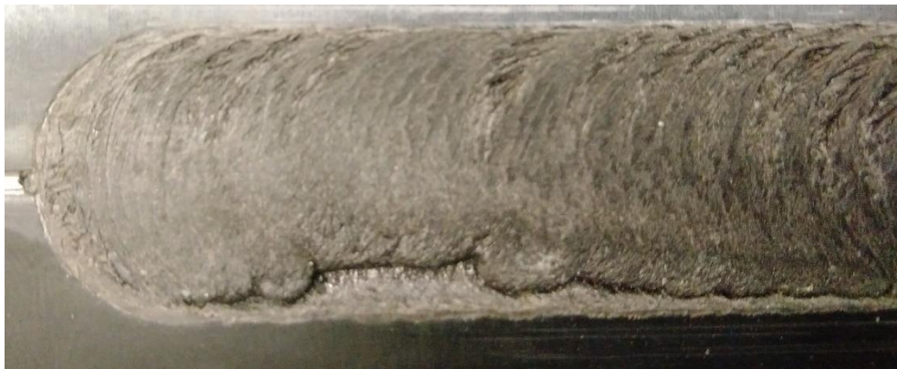
Figure 56 - Defect in the retreating side and onion ring defect of the surface of weld.
