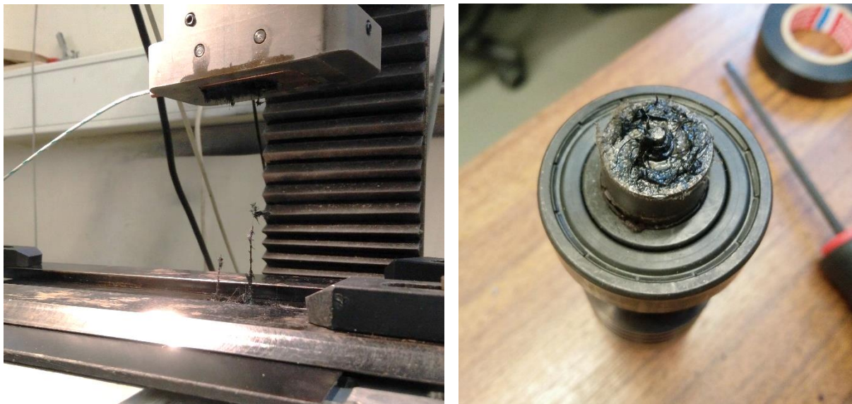
Figure 54 - Weld material stuck inside the tool, on the probe and on the shoulder face
