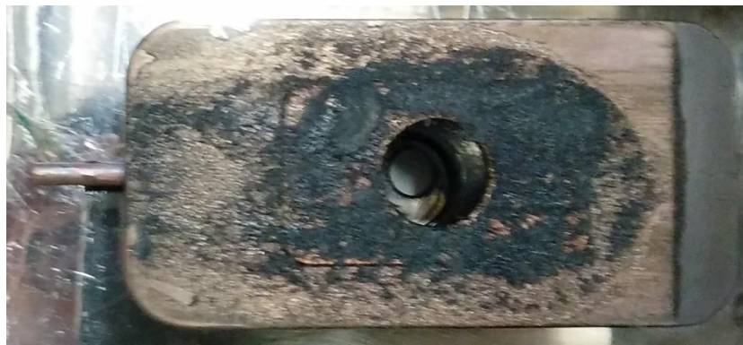
Figure 71 - Weld material stuck to the bottom of the welding tool
