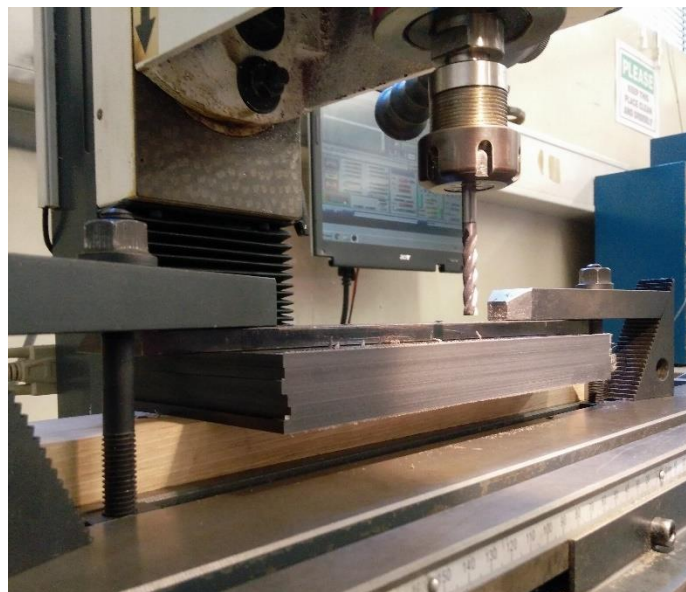
Figure 35 - Machining of the edges of 4 plates
