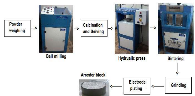
FIGURE 6. The production process of arrester blocks.
