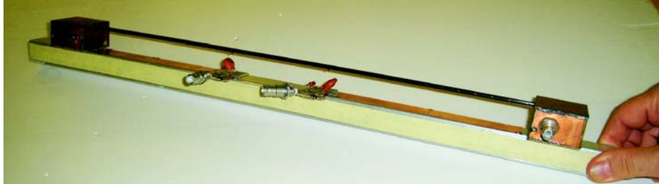
Fig. 4. Straw 4 mm in diameter and about 465 mm long with three anode segments
