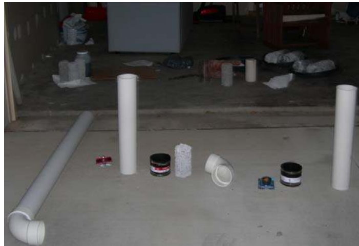
Figure 4.6: Materials Used for Falling Head Permeability
