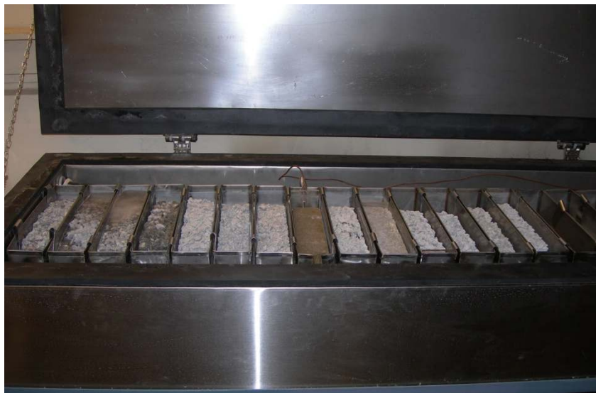
Figure 4.8: Specimens in Freeze-Thaw Chamber
