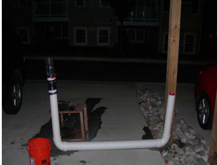
Figure 4.7: Assembled Falling Head Permeability Test
