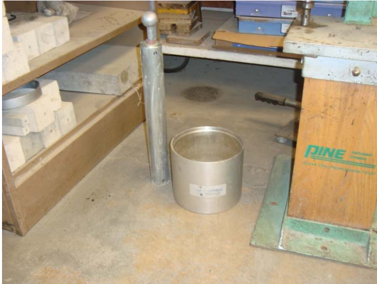
Figure 4.1: Apparatus Used for Density and Void Content
