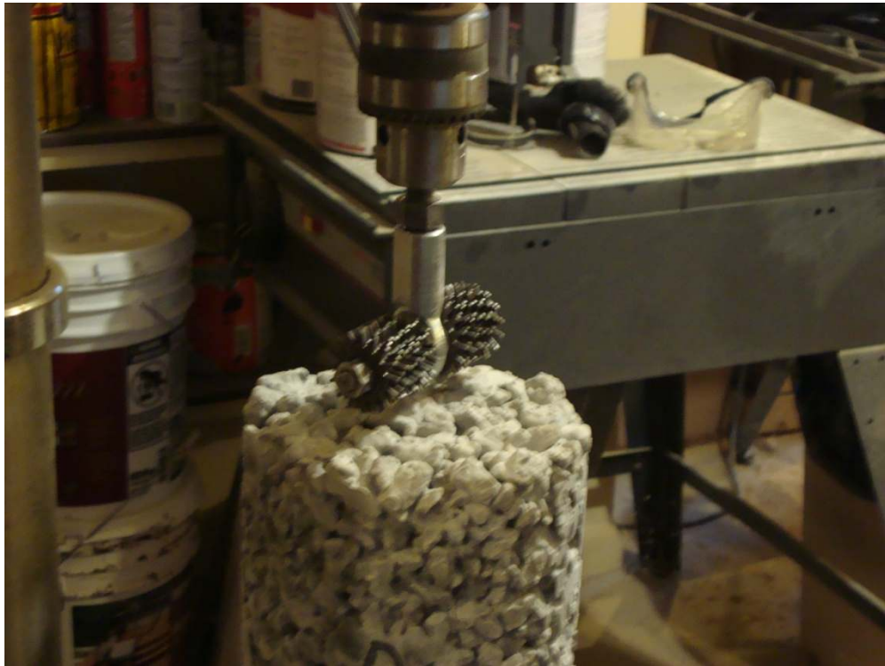
Figure 4.12: Surface Abrasion Test
