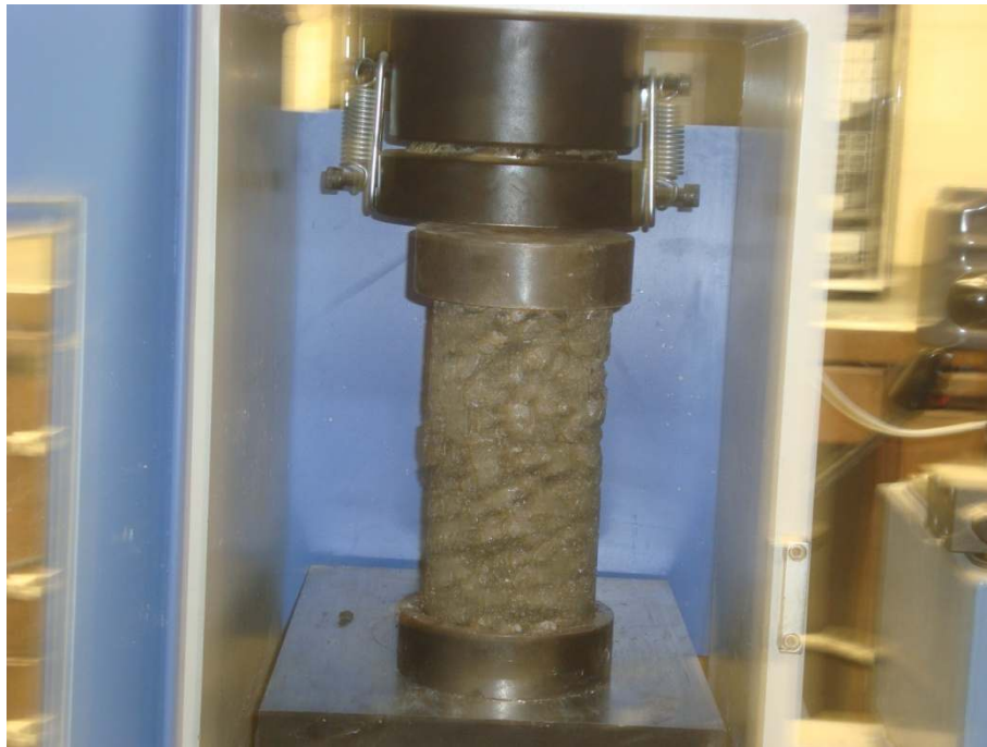
Figure 4.2: Pervious Concrete Specimen in Compression Testing Machine
