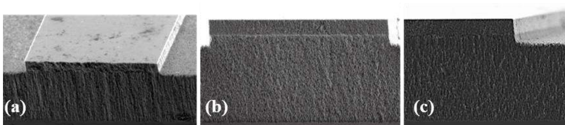
Fig. 5.14. FE-SEM image of the 10µm-wide access waveguide: (a) 60°-sectional image; (b) cross-sectional image; (c) cross-sectional image with lateral view.
