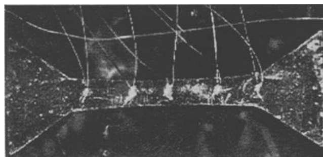
Fig. 3—A stainless steel microsample with five type-K thermocouples placed across its gage section. Thermocouple wires are 12 \mu\text{m} in diameter
