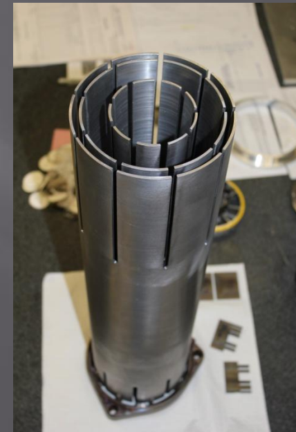
Spiders with baffles for 5 (4 + 1 spare) flight and 1 qual units
