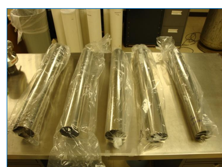
60 cm length – 5 cm diameter - 250 μm thick
