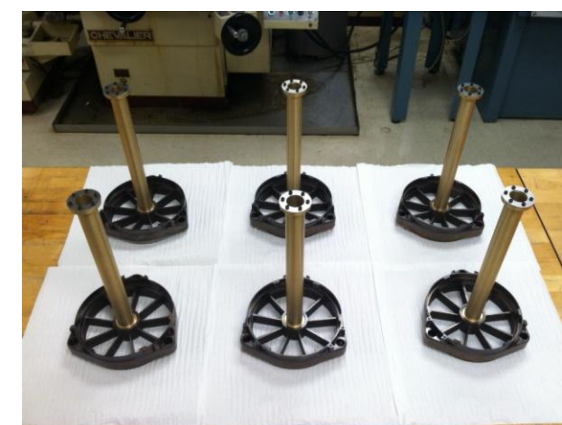
Spiders with baffles for 5 (4 + 1 spare) flight and 1 qual units
