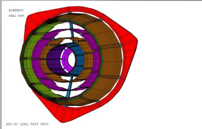
3 mass simulators and 6 shells installed on the spider
