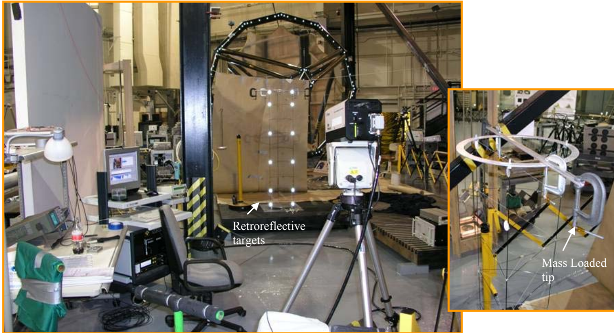
Figure 10. Mast Modal Test – General Set-up
