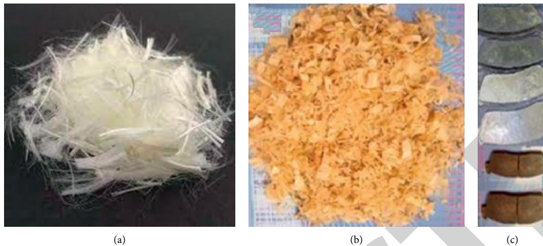
FIGURE 1: (a) PAN fibre. (b) Raw material of mulberry fibre. (c) Developed brake pads of mulberry-PAN fibre.
