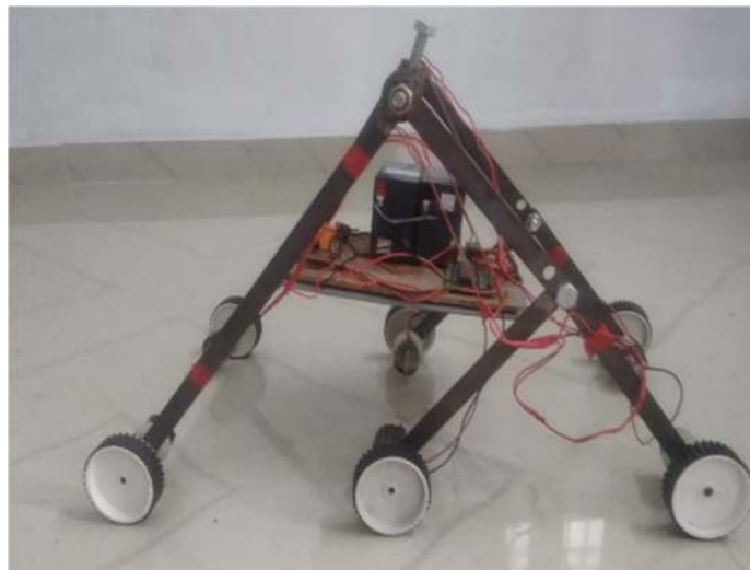
Fig6: Stair climbing: Expanded mode
