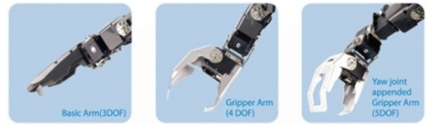
Fig. 5. Different types of grippers for DARwIn-OP
