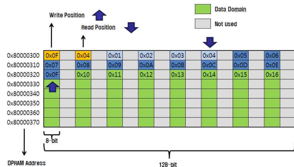
Fig. 3. DPRAM ring buffer structure
