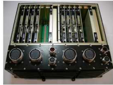
Fig. 2. Flight control computer of Smart UAV
