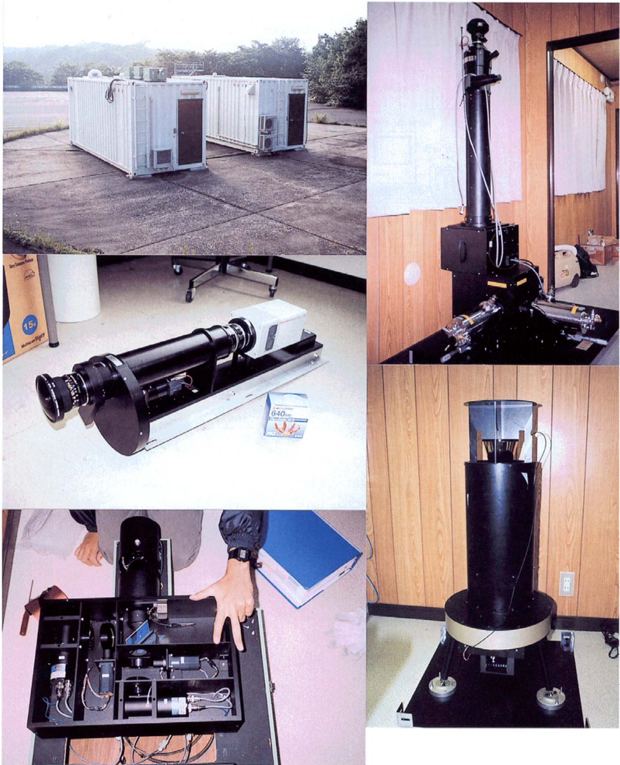
Fig. 2. Pictures of the instruments of OMTI. Two container houses (top left) with three photometers and several transparent domes on the roof, an all-sky camera (middle left), a meridian-scanning tilting photometer (bottom left), an imaging Fabry-Perot interferometer (top right), and a Spectral Airglow Temperature Imager (SATI, bottom right).
