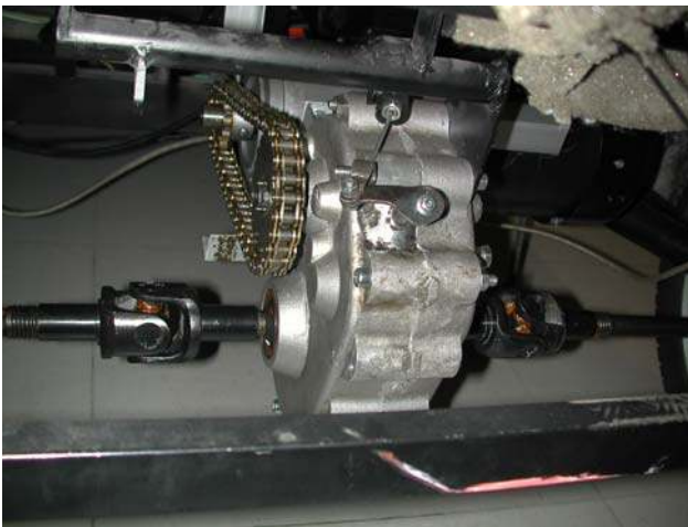
Fig 5.7: Gear and universal joint of the EV
