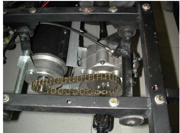
Fig 5.8 Motor and the step down gear
