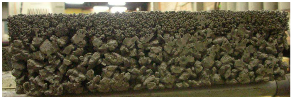
Figure 3.6 Specimen of pervious pavement system
