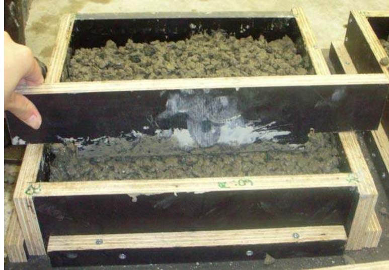
Figure 3.8 Casting of combination of pervious concrete and mortar
