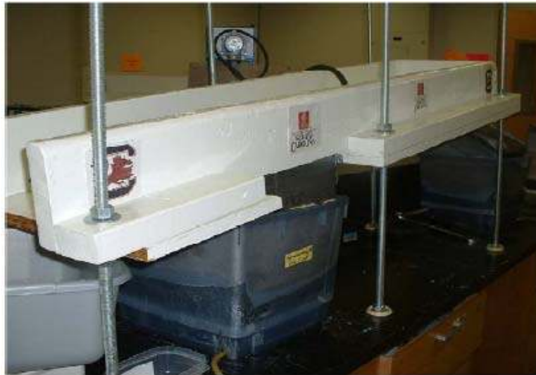
Figure 2.24 Experimental set-up for clogging test [17]
