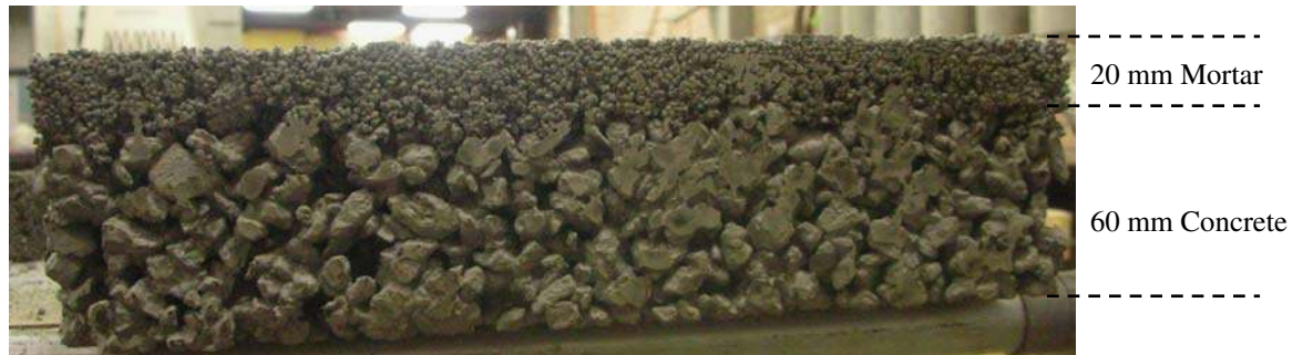
(a) Combination of pervious concrete and mortar Mix PCM1
