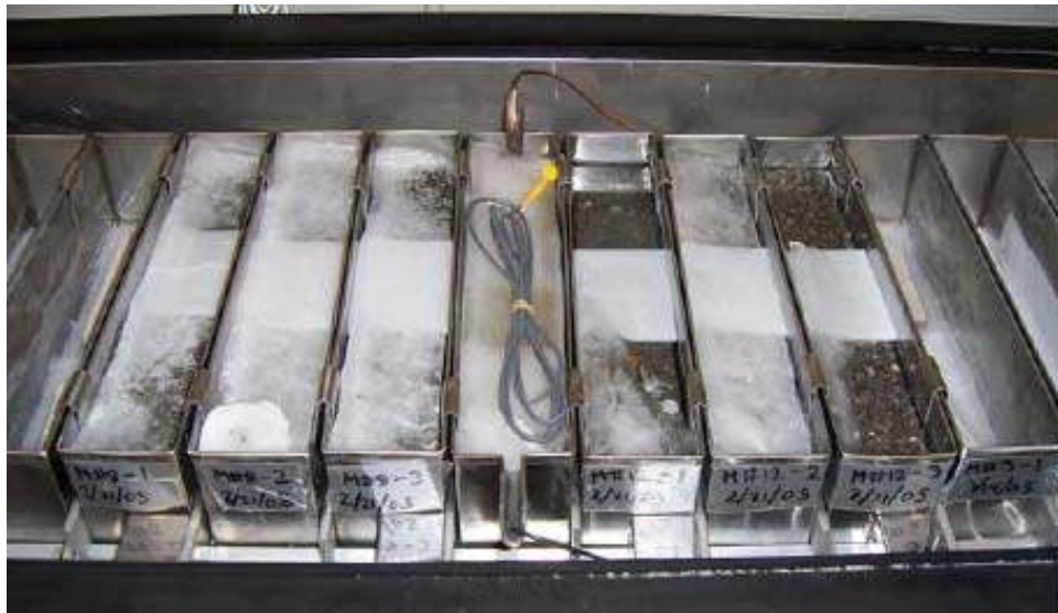
Figure 2.20 Freeze-thaw resistance test for pervious concrete [32]
