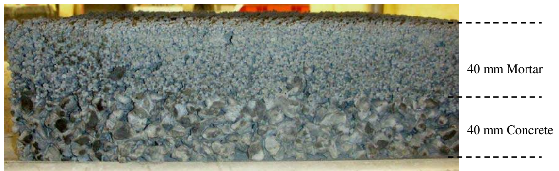
(b) Combination of pervious concrete and mortar Mix PCM2
