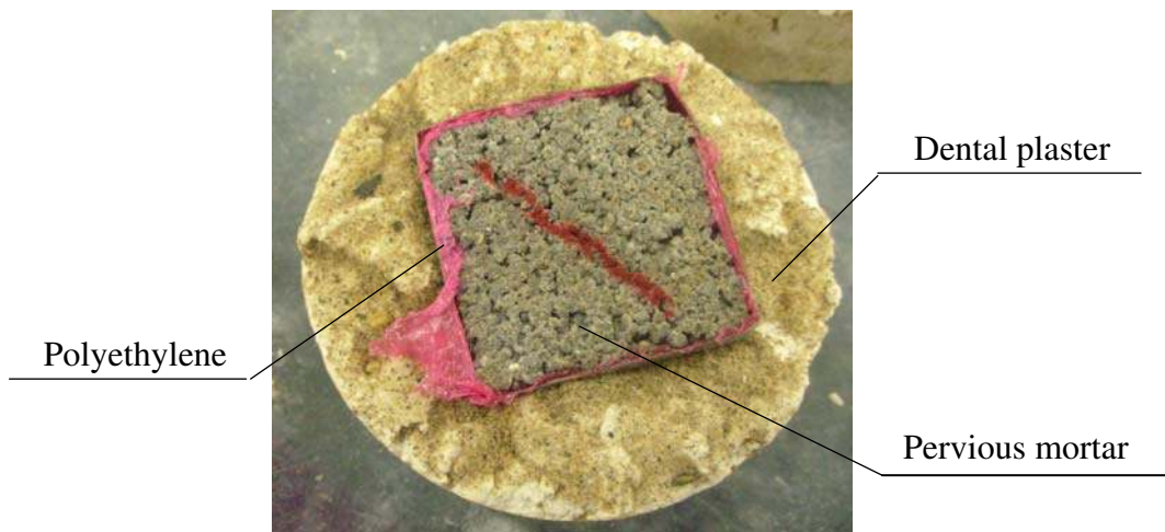
Figure 3.10 Pervious mortar specimen for water permeability
