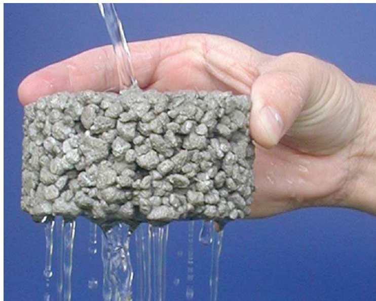
Figure 1.2 Pervious Concrete block [7]
