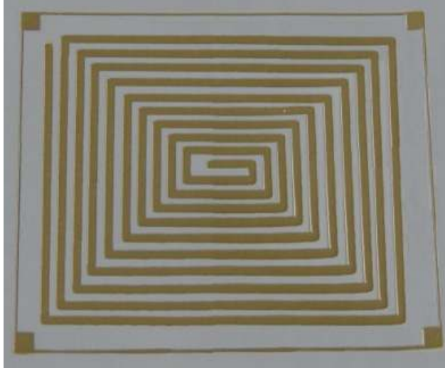
Figure 8.17 Implementation of Inductor windings on LTCC
