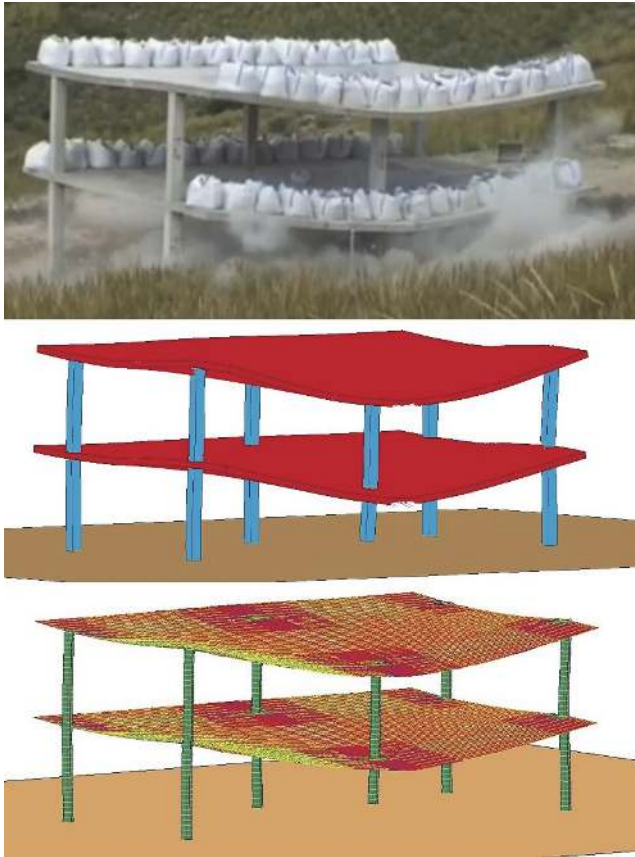
FIGURE 10: Comparison between test, continuum model, and structural model at 0.6 s after column removal.
