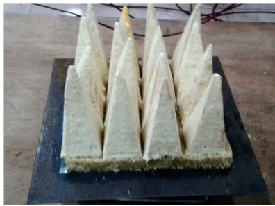
Figure 5. Single units of the SCB pyramidal microwave absorber after fabrication using a pyramidal-shaped mold.
