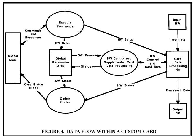
is executed, a response is generated and it is placed in the global memory buffer by the command handler. When all commands are executed, the master is notified that a response is available.
