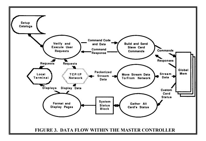
The path through the center the figure #3 represents the use of a remote device as a source or destination of telemetry data. Remote data stream transfer is handled by a separate task. This process picks up the data from a global memory buffer and transfers it to a remote device on the network or vice versa using the network communications software. The remote data transfer task can run on a separate processor dedicated to its function if needed.
