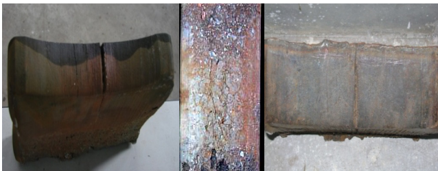
Figure 3. Typical cracks observed on the rolled blooms
