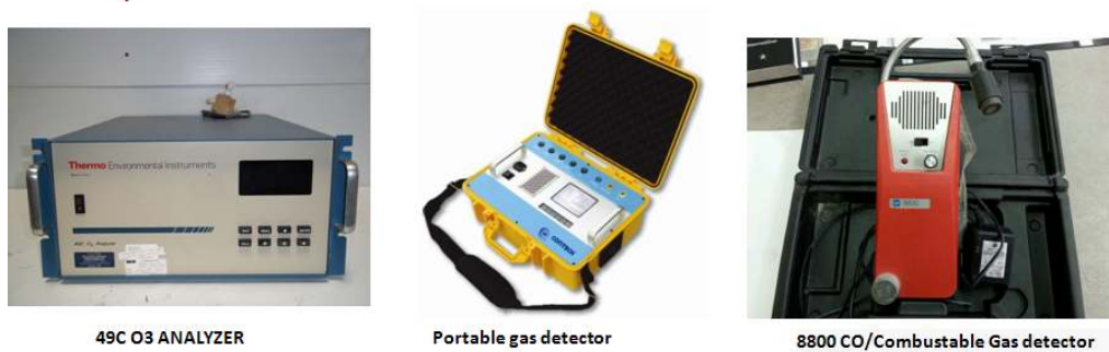
Figure 1: various portable environmental monitoring instruments.
