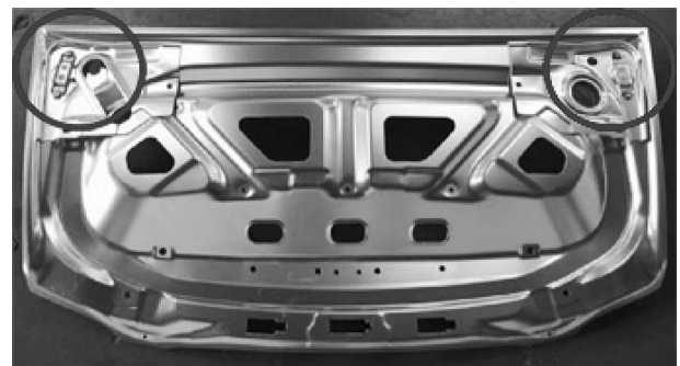
Fig. 8 SFW of aluminum to steel used in an aluminum trunk lid.
