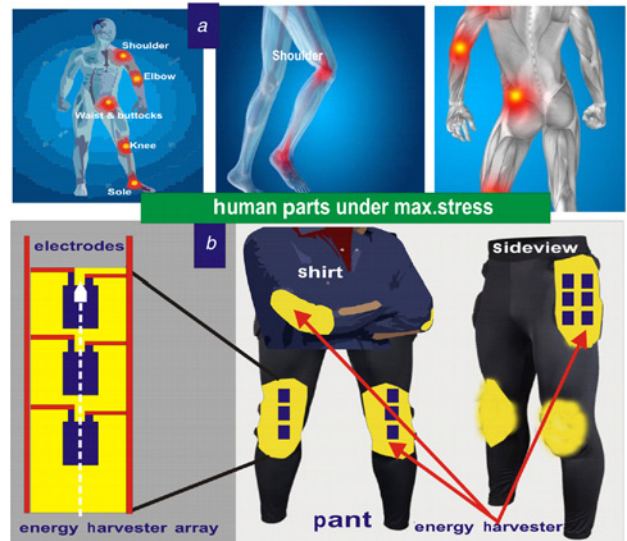
Fig. 3 Identified spots based on optimum level of stresses a Prominent energy hot spots b Energy Harvesting mounting
