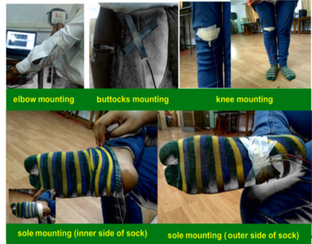
Fig. 12 EHD mounting on energy hot spots
