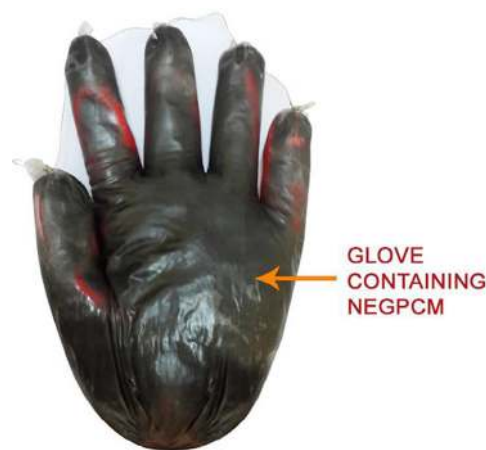
Fig. 4. Photograph of nano eutectic gel phase change material (NEGPCM) composite based hand glove, with ultrafast charging characteristics, developed for use in higher altitudes where less sunshine occurs/where is no external power available.
