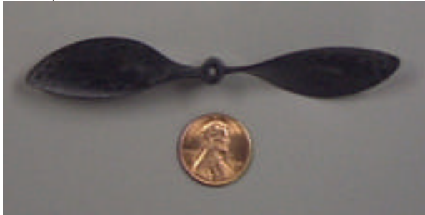
Figure 6: Micro-propeller designed for 4:1 gearbox
