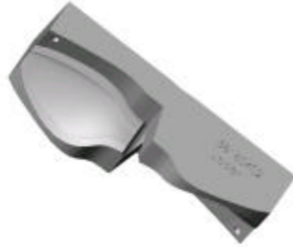
Figure 7: Upper half of propeller mold
