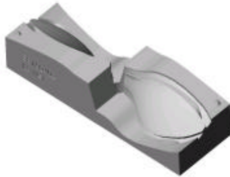
Figure 8: Lower half of propeller mold
